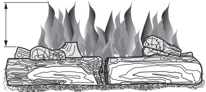
Figure 31 - Incorrect Burner Flame Pattern (Actual logs will vary from illustration.)
