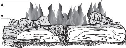
Figure 30 - Correct Burner Flame Pattern
