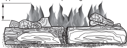
Figure 29 - Correct Burner Flame Pattern
