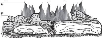
Figure 21 - Correct Burner Flame Pattern
