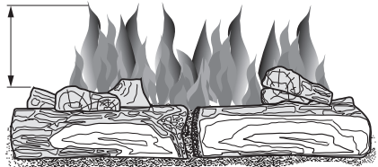
Figure 22 - Incorrect Burner Flame Pattern
