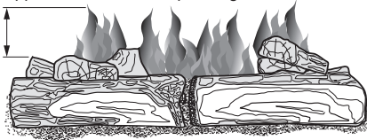
Figure 27 - Correct Burner Flame Pattern
