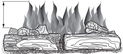
Figure 28 - Incorrect Burner Flame Pattern
