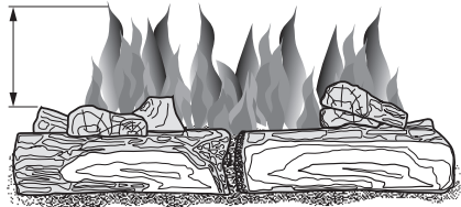
Figure 29 - Incorrect Burner Flame Pattern
