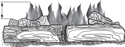
Figure 28 - Correct Burner Flame Pattern
