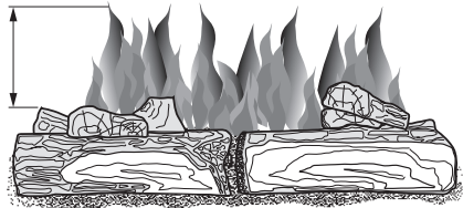
Figure 29 - Incorrect Burner Flame Pattern
