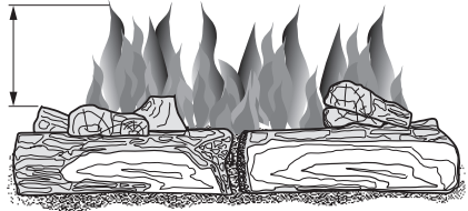
Figure 25 - Incorrect Burner Flame Pattern with Control Knob Set to HI (5)
