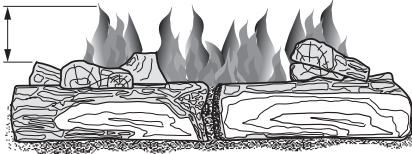
Figure 26 - Correct Burner Flame Pattern with Control Knob Set to HI (5)
