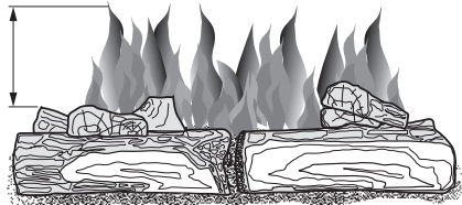
Figure 33 - Incorrect Burner Flame Pattern
