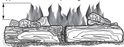
Figure 25 - Correct Burner Flame Pattern
