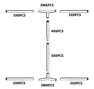
**1)** Start by laying out all of the parts and pieces to your King Canopy. Please refer to the parts list to ensure that your kit is complete. When all the parts have been accounted for, begin to layout your frame according to the photo above (5X0PCS & 4X6PCS). Each 3-way fitting (3WAPCS) should be placed at the two end peaks.
