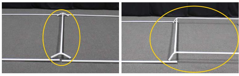
**2)** Now that all the pipe and fittings are laid out as displayed in the photo, begin to connect the center pipe and fittings. Start assembly by working from one end to the other, connecting the center ridge pipe into the 3-Way (3WAPCS) fittings.
