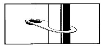
Curtain clips may have to be re-tightened occaisonally due to strong wind gusts. IMPORTANT! Once the legs and cover are assembled, your canopy will act like a kite in the wind. It is imperative that the canopy anchors be installed NOW!
