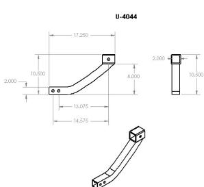
ATV/UTV Hitch 1 1/4" to 2" Hitch Riser/Extender/
