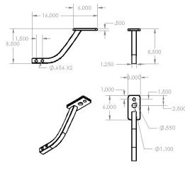
ATV/UTV Hitch 1/4" to 2" Hitch Adapter/Extender that features a very short extension;4.5"If you'd like to go directly to this
