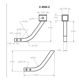
ATV/UTV Hitch The Hornet U-4044-FP is an ATV/UTV 1 1/4" Hitch Riser/Extender that features a tow plate with 2 holes; one for a ball hitch and the other hole can accommodate a yard cart or other trailer with a y hitch.
