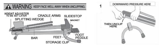
UNIT COMES IN TWO PIECES. ASSEMBLY REQUIRED. TAKEOUT STORAGECLIP, THEN SLOWLY RELEASE PRESSURE. THEBAR WILL RISE TO 2 INCHES.
