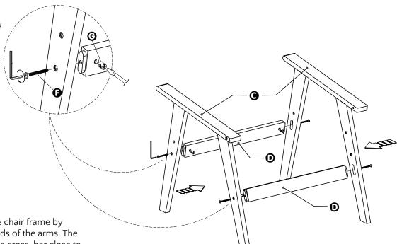
2 Identify the front of the chair frame by finding the rounded ends of the arms. The *front* of the **Seat** has the cross-bar close to the edge, and the *back* has longer ends on the side bars.
