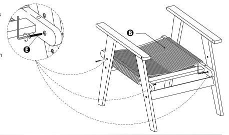
To install the Backrest (a), insert the tenons at the bottom of each end of the Back into the mortises in the top of the back end of the edge pieces of the seat.
