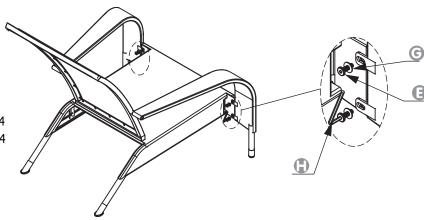
Attach the Arms ③ and ⑤ to the Seat Back ⑥ by sliding the arms onto the pegs on the sides of the Seat Back, then using a Bolt ⑤ with a Washer ⑥ to fasten each Arm as shown. Tighten using the Hex Wrench ⑥.
