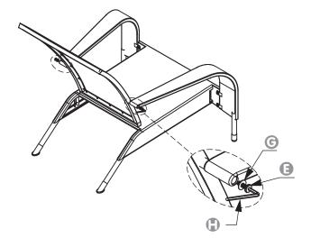
Attach the Seat ① to the Seat Back ② using 3 Bolts ① with Washers ②, inserted through the Seat and into the Seat Back. Tighten using the Hex Wrench ①.
