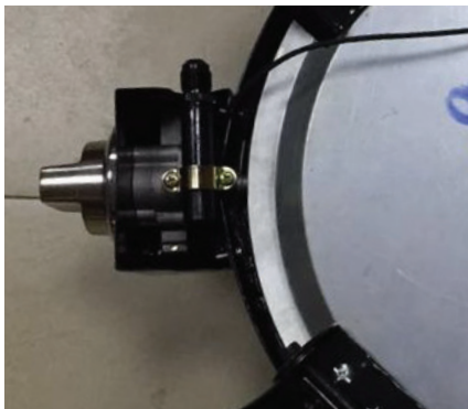
Underside of Burner
