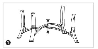
Place the Fire Bowl Assembly D upside down, and fix Leg Assembly to Fire Bowl with four M6x10 Wing Screws ().
