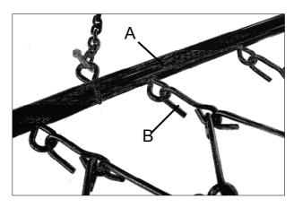
2. Connect rear, harrow section B to front, harrow section C.
