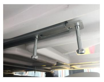
3. With the flat brackets assembled ,lift the side of the RTT and slide 2 flat brackets with bolts along each mounting rail. Slide the flat brackets with bolts along the mounting rails
