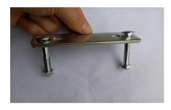
2. Assemble 4 of the flat brackets with 2 bolts each.
