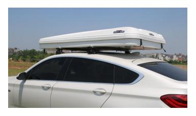
1.Lift the RTT onto your vehicle's roof rack.Position so that the weight is centred evenly over the roof.
