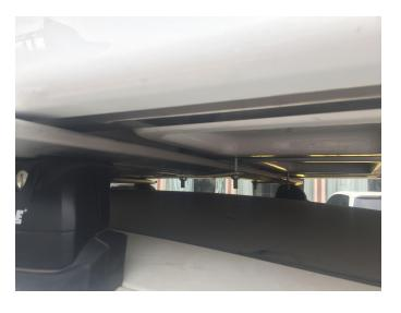
4. Connect the 4 remaining flat brackets with 2 nuts each. Tighten all the nuts, making sure the RTT is firmly mounted and will not move. The flat brackets should have a slight bend around the cross bar .
