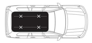
5. The RTT should have 4 spaced ,strong points of contact on the roof rack.
