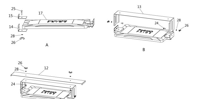
• Hang the Heater group on top of the Frame. Fix the Hook Bolt as below diagram for hanging the hearter wire.
