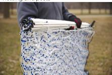
**3.** While holding the posts, walk backwards and lay out one post at a time; unfold the entire roll of netting.
