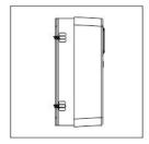
step5:Fasten the controller into the pilot screws
