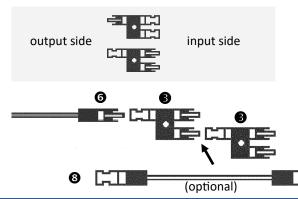
With the other 15-ft MC4 cable **⑤**, connect one branch connector **⑤** with the "male" output to the "female" end of the cable. Connect an additional "male" output branch connector **⑤** to the attached branch connector.
