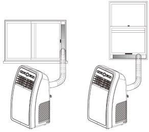
Ensure that the exhaust hose remains as straight as possible. A bent or curved exhaust hose will not work efficiently.
