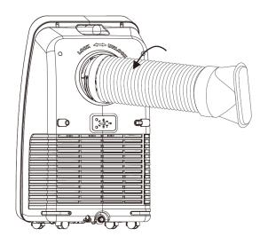
Insert the exhaust hose into the window sealing plate, and adjust the opening of the window so that the sealing plate fits in the window properly. (Note that the length of the sealing plate is adjustable)
