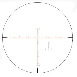
The new Top Angle 7-30X50mm MOA scope features a new MOA reticle for precision shooting. The Center features a 1/16 MOA dot. The center opening measures  $\frac{1}{2}$  MOA by  $\frac{1}{2}$  MOA. Both the horizontal and vertical axes indicate quarter MOA subtensions.
