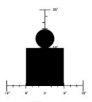
Both of these targets are properly framed in the ranging scale. Notice how the width of the silhouette roughly measures 18" and the total height of the silhouette measures 27". If the target you are trying to frame is too small, increase the magnification. If the target you are trying to frame is too large on the scale, reduce the magnification.
