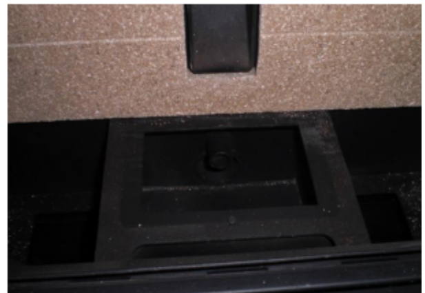
Figure 32: Burn Pot Cradle/Igniter Tube
