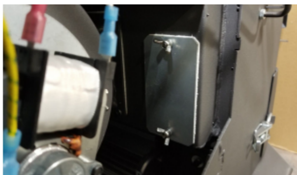
Figure 33C: Exhaust Chamber Cover Plate. Exhaust side (2)
