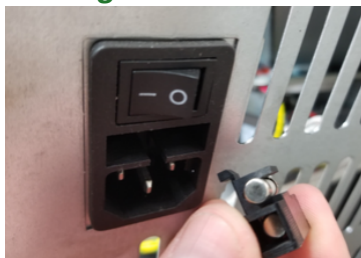
Figure 20B: Spare Fuse
