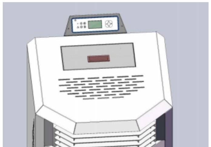
Figure 18: Control pad location
