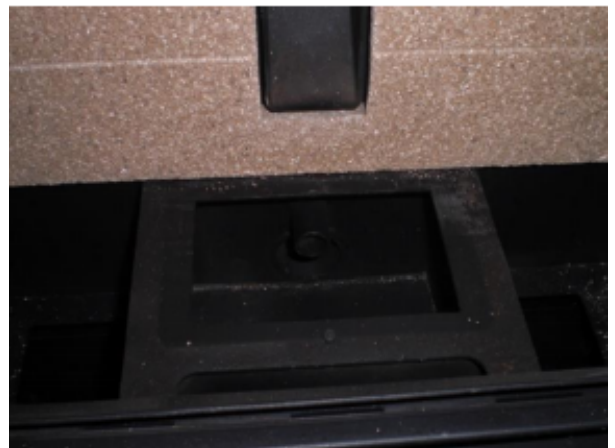
Figure 32: Burn Pot Cradle/Igniter Tube
