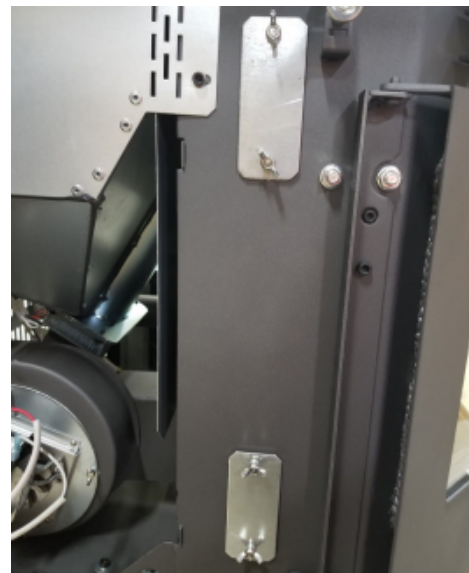
Figure 33B: Exhaust Chamber Cover Plates. Exhaust side
