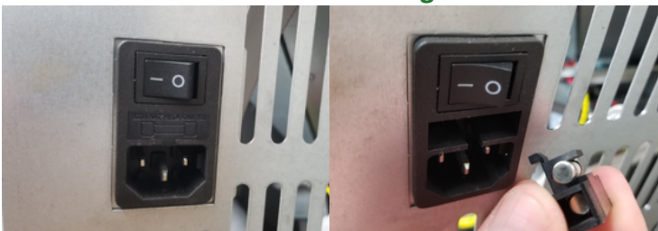
Figure 20A: Power Switch Figure 20B: Spare Fuse
