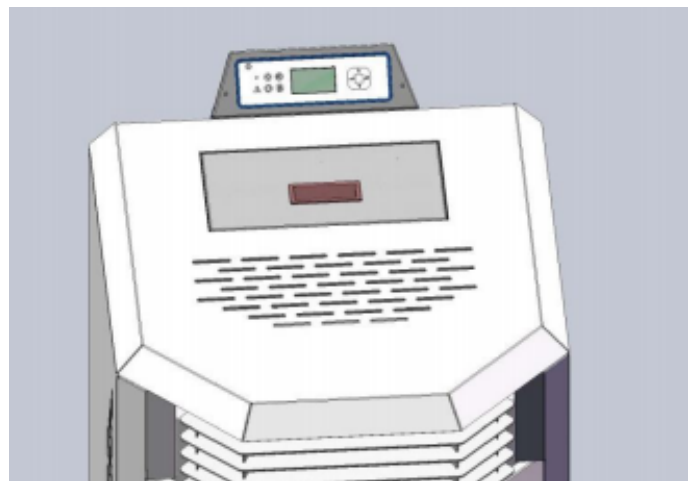
Figure 18: Control pad location
