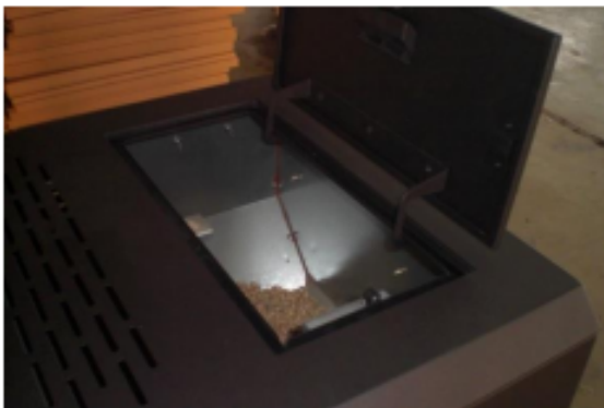
Figure 21: Pellet Load Hopper Lid
