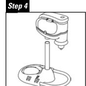
Completed assembly should have the front of power head in the same direction as base U-shaped legs.
