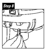
Plug power connector into the trap power slot located on the back of the power head.
