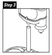
Place trap power head onto pole. Press down firmly with two hands to secure.
