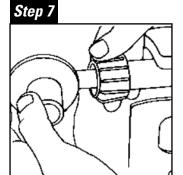
Making sure propane tank is fully closed, attach propane regulator hose to propane tank. Secure tightly by hand. Do not use tools.
