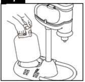
Place the base of the propane tank into the molded cradle supplied.
