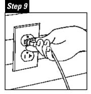
Plug Adapter into properly grounded electrical outlet.
