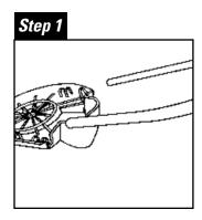
Place base upside down on a flat surface, slide U-shaped support legs into slots on base until they lock in place.
