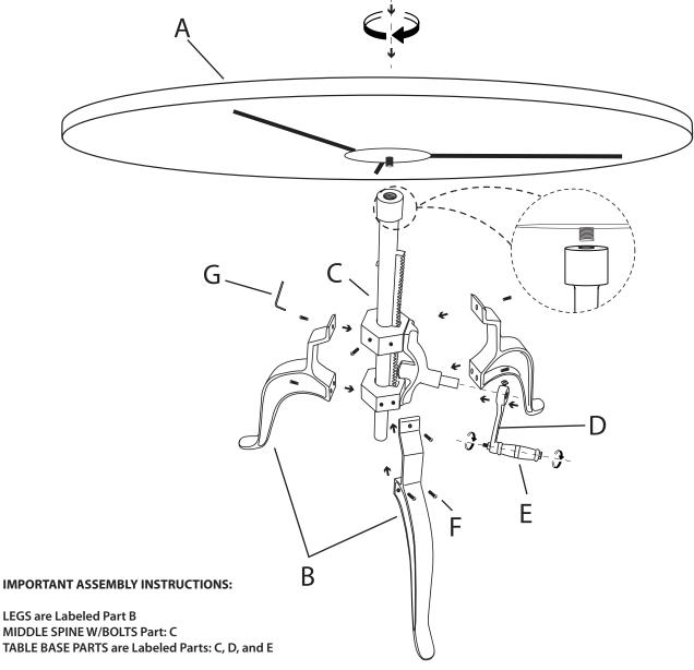
EACH LEG WHEN BEING ATTACHED REQUIRES TOP MIDDLE BOLT SPINE TO BE TIGHTENED BEFORE BOTTOM BOLTS ARE TIGHTENED
