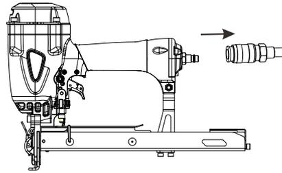
2. Turn the tool so the air inlet is facing up. Place 2 - 3 drops of pneumatic fastening tool oil into air inlet. Do not use detergent oils, oil additives, or air-tool oils as these lubricants will cause accelerated wear to the seals and bumpers in the tool, resulting in poor tool performance and frequent tool maintenance.
