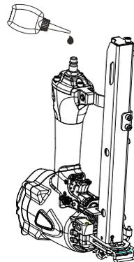
3. After adding oil, connect the tool to the air source, run tool briefly. Wipe off any excess oil from the cap exhaust.
