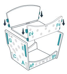
Fold the three-panel main seat section into a "U" shape and attach it to the left and right walls, matching the letters on the tabs and slots. The smooth side should face upward. Press down on the main seat section to lock it in place.
