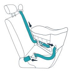
Pass your vehicle's seat belt through the slit at one side of the safety seat, through the seat belt tether loop, through the slit on the opposite side of the safety seat and buckle it.
