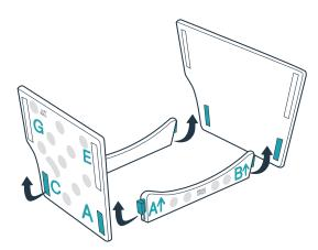
Attach the front and rear struts to the left and right walls of the safety seat frame, matching the letters on the tabs and slots. The smooth sides should face inward. Press up on each strut to lock it in place.
