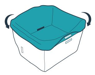
Insert the liner into the safety seat, lining up the slit in the liner with the back of the safety seat. Fold the liner over the edges and press the hook and loop fasteners together.
