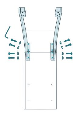
First, attach the legs to the top platform using four screws and washers. Next, attach the legs to the middle platform using four screws and washers. Wait until all the screws are in place before you tighten them.
