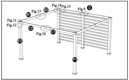
Attach the beam cover plate (O) to the assembled back beam(D1/D2) with bolts (AA) and flat washer (BB). Tighten with allen key (Z1).
