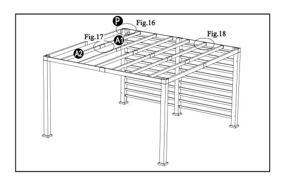
16. Attach the corner cover plate (P) to the short beam short side (B1) and long beam short side (B2) with bolts (AA) and flat washer (BB).
