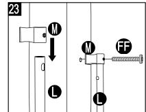
24. Attach the cloth tube connector (M) to the cloth tube (L) from bottom and then secure with bolts (FF). Tighten with allen key (Z1).
