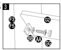
Connect the bottom decoration tube (G2) to the post (F4) with bolts (AA), flat washer (BB) and cover plastic cap (GG). Tighten with allen key (Z1).
