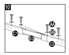
Attach the assembled front beam (C1/C2) to the Post (F1/F2) with bolts (AA), flat washer (BB) and spring washer (CC), assemble from inside direction. Then cover with plastic cap (GG). Tighten with allen key (Z1).
