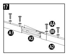
18. Attach the assembled short trabecular (A1/A2) to the back left beam (D1),back right beam (D2), front short beam (C1) and front long beam (C2) with bolts (AA) and flat washer (BB).Then cover with plastic cap (GG).Tighten with allen key (Z1)
