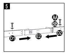
Attach the assembled back beam (D1/D2) to the post (F3/F5) with bolts (AA), flat washer (BB) and spring washer (CC), assemble from inside direction. Then cover with plastic cap (GG). Tighten with allen key (Z1).
