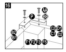
17. Connect the short trabecular A1 and A2 to the trabecular connector (A3) with bolts (AA) and flat washer (BB). Tighten with allen key (Z1).
