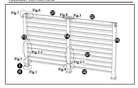
1. Attach the base cover (I) to the post (F1/F2/F3/F4/F5). Then attach the base (H) to the post with bolts (AA) and flat washer (BB). Tighten with allen key (Z1).
