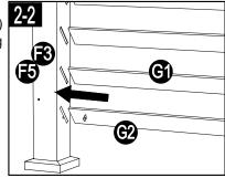
3. Connect the bottom decoration tube (G2) to the post (F3/F5) with bolts (AA) and flat washer (BB). Then cover with plastic cap (GG) .Tighten with allen key (Z1).
