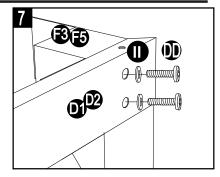
8. Connect the assembled back beam (D1/D2) to the post (F4) with bolts (DD) and washer (II). Tighten with allen key (Z1).
