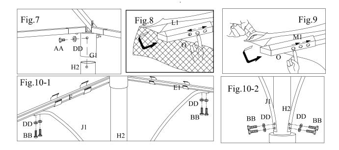
**Fig.7:** Lift assembled roof (G1) up, fix connector (G1) and post (H2) with bolt (AA), flat washer (DD) Repeat for all posts. (Fig8).
