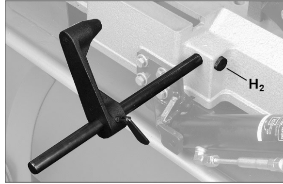
Figure 6-7: installing work stop (712 only)
