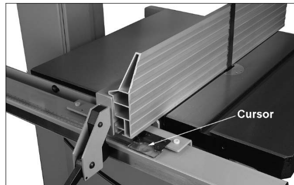
Figure 12: calibrating fence cursor
