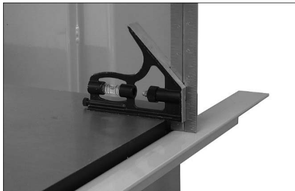
Figure 5: aligning rear rail
