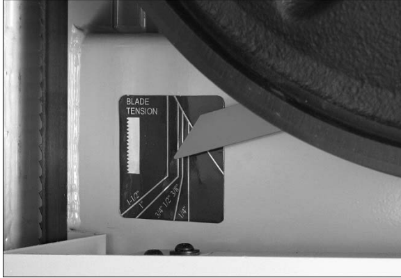
Figure 25: blade tension scale
