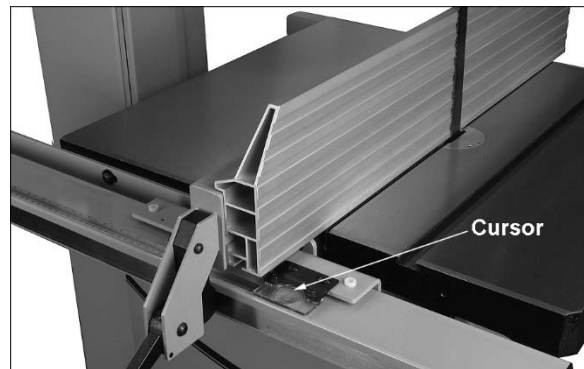
Figure 12: calibrating fence cursor
