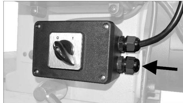
Figure 7-1: main switch box
