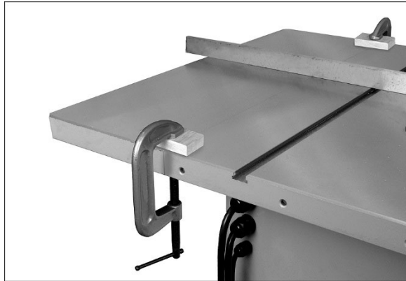
Figure 6-5: leveling extension wings, method 2
