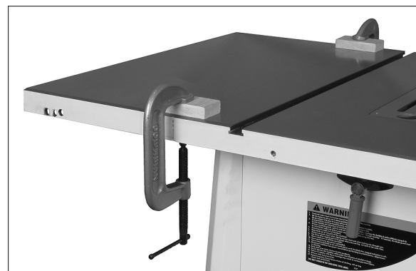
Figure 6-6: leveling extension wings, method 2
