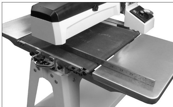
Figure 6-4: extension table alignment
