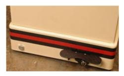
The 1½ HP motor (left) has plenty of power for planing and molding operations. Wheels built into the base cabinet (right) make moving the machine easy. The pedal locks and unlocks the wheels.
