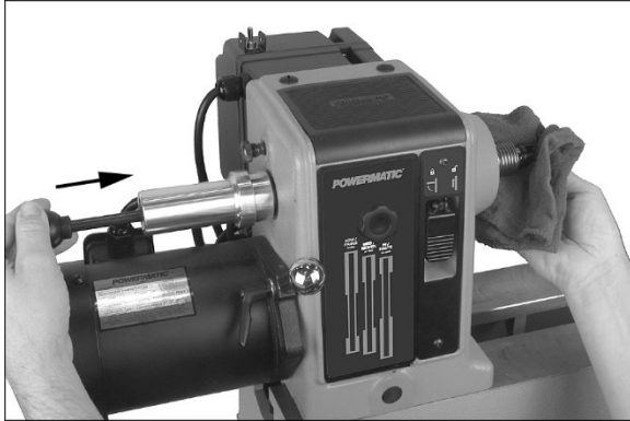
Figure 8-5: removing center from headstock
