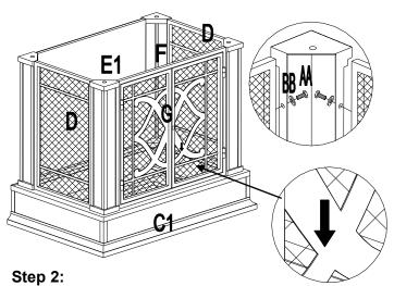
Place Rear Board (E1), Side Mesh (D) and Door (G) between two Posts (F), and use 16pcs Bolts and Flat Washers. Fasten with Wrench (DD). Do not tighten now. Place the door as the arrow direction
