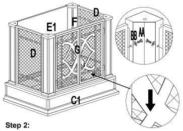
Place Rear Board (E1), Side Mesh (D) and Door (G) between two Posts (F), and use 16pcs Bolts and Flat Washers. Fasten with Wrench (DD). Do not tighten now. Place the door as the arrow direction
