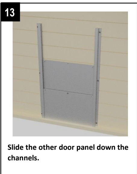
It must be in the second slot in each channel. The screws and nuts must be at the front.
