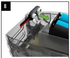
Fit the connector to the battery
