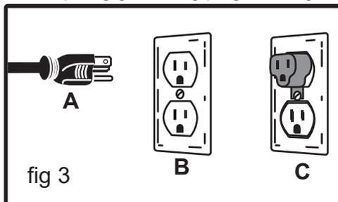
type receptacle (B, fig 3). Do not remove the 3rd prong (grounding pin) to make it fit into an old 2-hole wall socket or extension cord. If an adaptor plug is used (C, fig 3) it must be attached to the metal screw of the receptacle.
